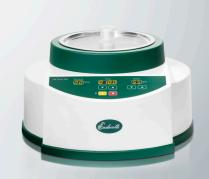
The new Air Sizer 200 is ideal for sieving very fine dry particles, which require efficient dispersion and desagglomeration via air jet technology (e.g. electrostatic material).
